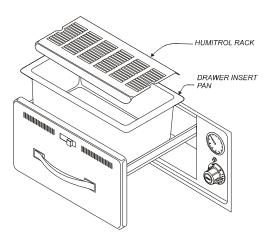
Fig. 8 Roll Warmer Drawer Pan Installation
